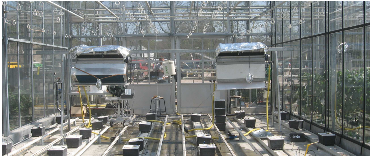
Figur 10. Measuring system for the PTC + with the OPAC106 heat exchanger in parallel with the FiWiHex heat exchanger
